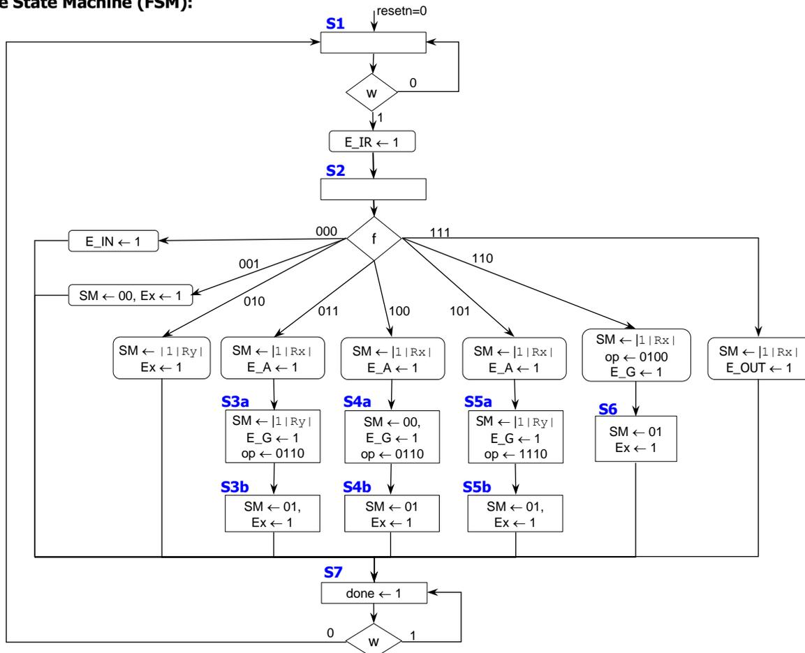
▪ **Decoder with enable:** This circuit simplifies the FSM diagram. A suggested code is listed below:
